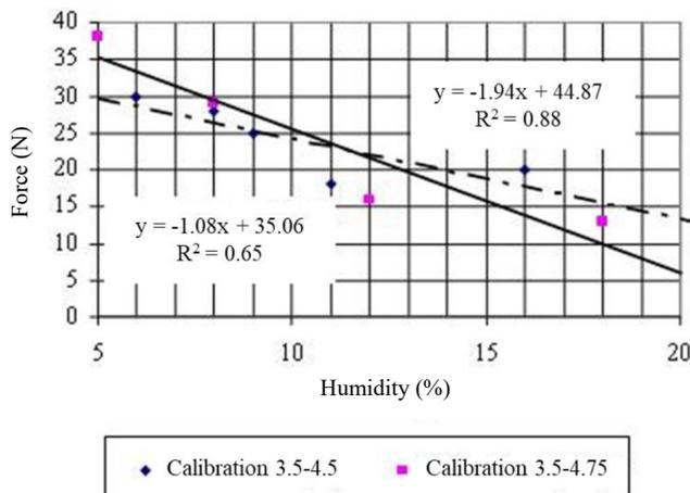
**Fig. 3.** Intensity of the destructive strength affecting the sugar beet seeds with a calibration of 3.5-4.5 and 3.5-4.75 mm.
