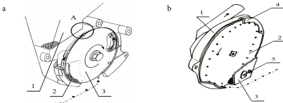
**Fig. 1.** Detail from the mechanical planting mechanism (Findura and Košičiarová, 2020) (a): 1 – bin for seeds, 2 – filling chamber, 3 – planting disc, A – disc picking hole. Detail of the pneumatic planting mechanism (b): 1 – vacuum chamber, 2 – planting disc, 3 – filling chamber with seeds, 4 – wiper, 5 – seed outlet.
